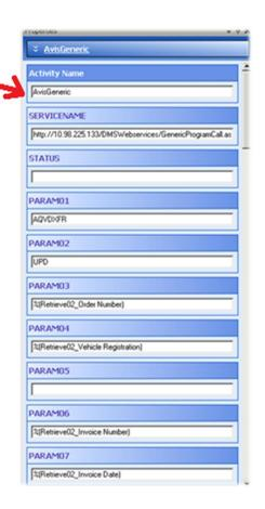
We basically call a Web Service by a specific path and pass the parameters into the FMS via the Web Service:
